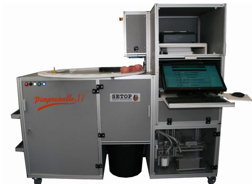
Figure 2.16 Pimprenelle II machine for quality analysis.
