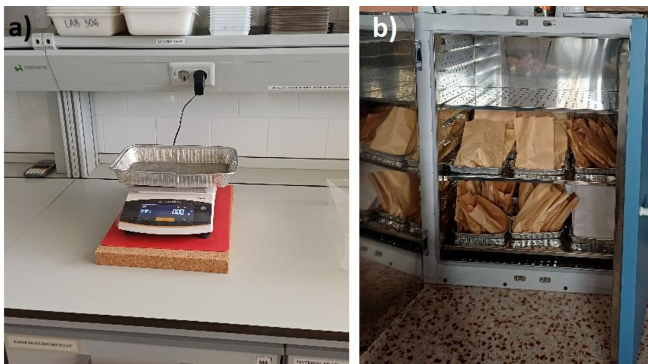
Figure 3.17 Equipment used for weight determination: a) precision balance for weight measurements and b) forced-air drying oven with labelled samples.
