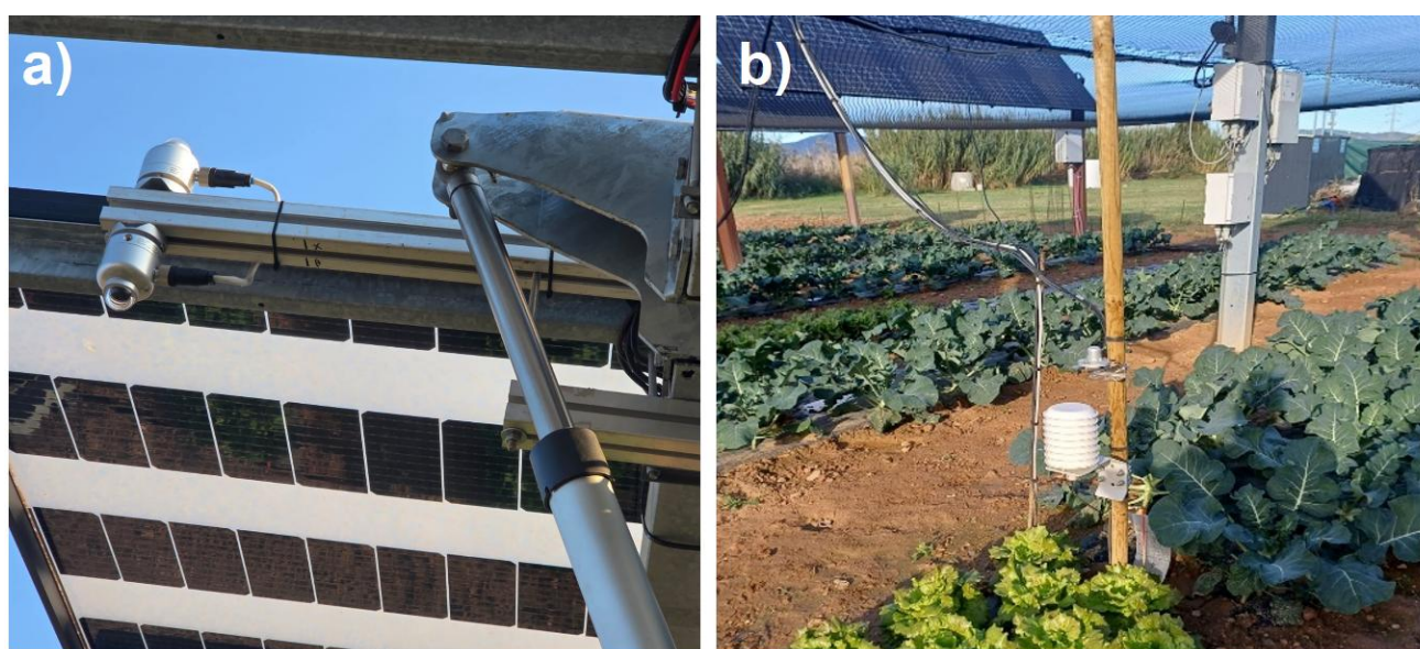
Figure 3.5 Environmental sensing in the agrivoltaic plots: (a) PAR radiation measurement; (b) soil monitoring at crop level.
