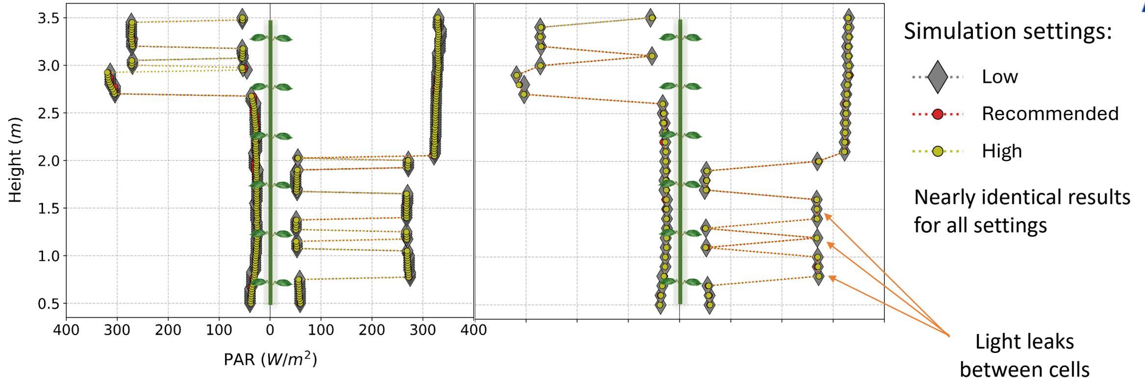
Lower spatial resolution with 10 cm spacing between sampling points (plot on the right) effectively captured light leaks between cells.
