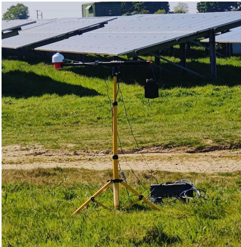
Figure 2.5: Ground Station setup used for global irradiance measurements
