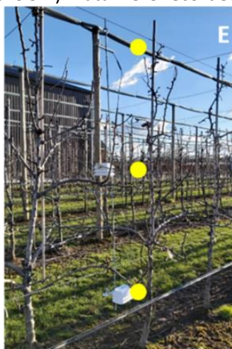
Figure 5.3 PAR sensor placement in 2024 [38]. Yellow dots indicate sensor heights ( h = 60, 150 and 250 cm).
