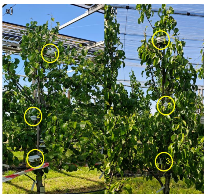
Figure 5.6 Temperature and humidity sensor placement in 2025. a) APV plot. Sensor height: 1 - approx. 265cm; 2 - approx. 155cm; 3 - approx. 100cm. b) FS plot. Sensor height: 1 - approx. 265cm; 2 - approx. 175cm; 3 - approx. 110cm.
