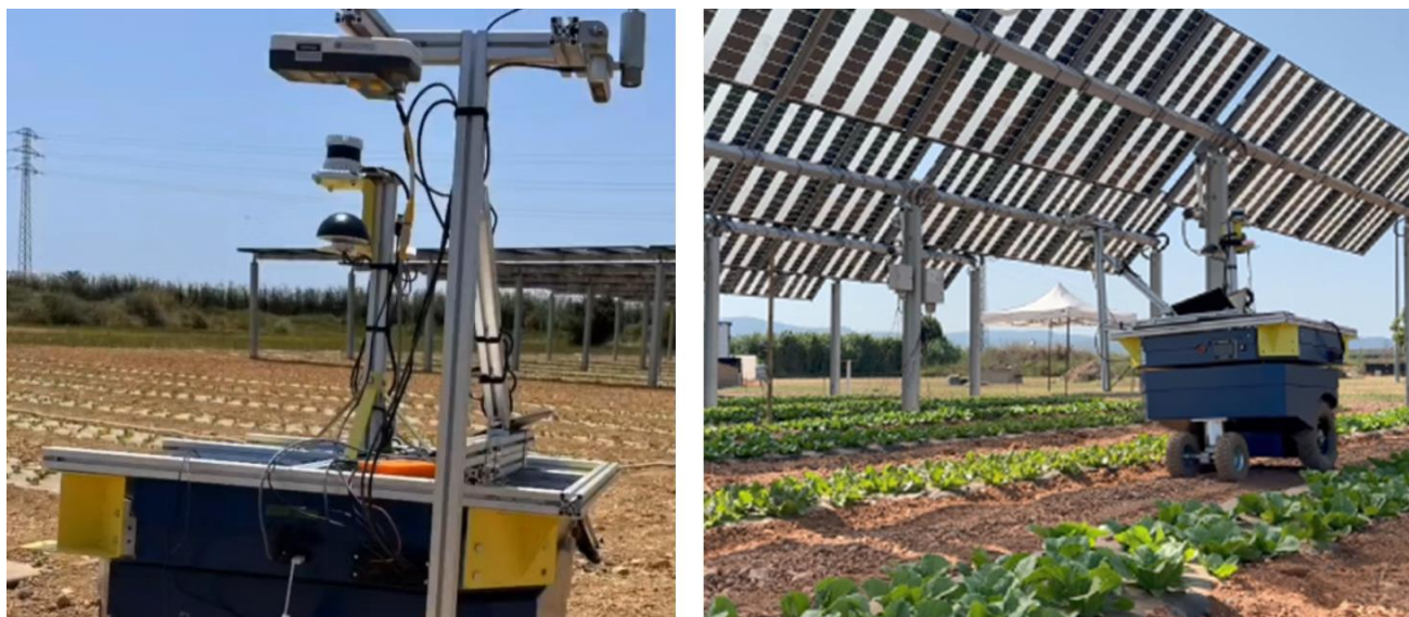
Figure 2.14: Left: Detail of the sensor suite mounted on the ground robot (RGB camera, thermal camera and Crop Circle sensor). Right: The robot performing agronomic monitoring
