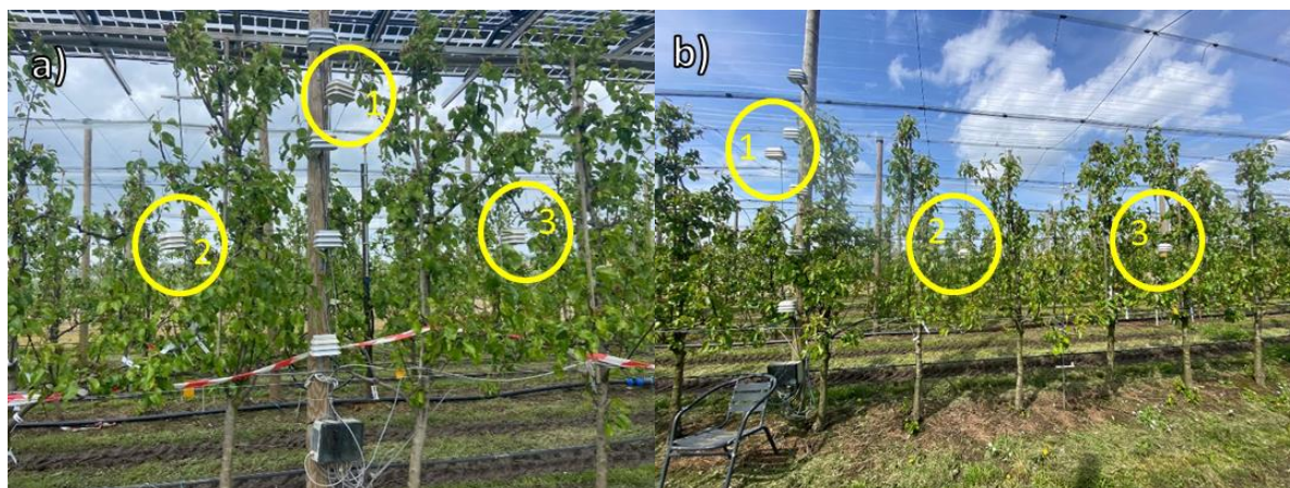
Figure 5.5 Temperature and humidity sensor placement in 2024. a) APV plot. b) FS plot. Height for the sensors: 1- approx. 250cm. 2&3 - approx. 150cm.
