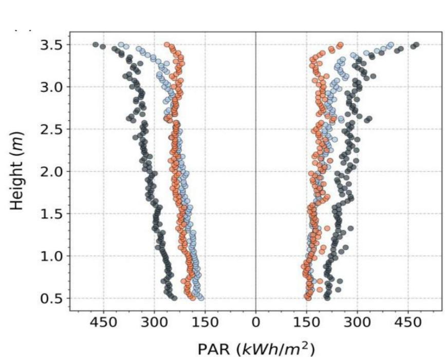
Seasonally aggregated profiles of light penetration through the tree canopy show that while overall patterns are similar to a reference orchard without PV, the presence of modules leads to a more uniform vertical distribution of photosynthetically active radiation (PAR) within the canopy.
