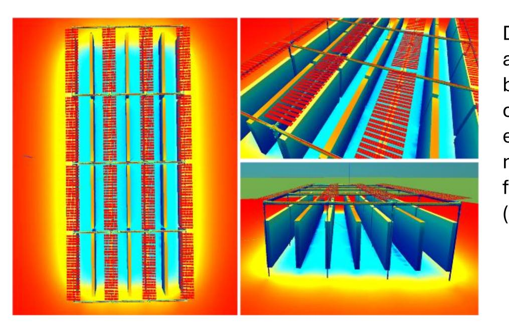
Distribution of diffuse irradiance across the full Agri-PV scene, based on sky visibility calculated from view factors at each point of the triangular mesh. Values are normalised from 0 (low visibility, in blue) to 1 (high visibility, in red).
