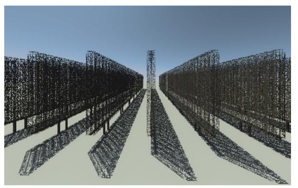
Modelling plant architecture is one of the most complex aspects of Agri-PV simulation, especially for tall, porous tree canopies that strongly influence light distribution. Instead of aiming for exact replication, simplified yet realistic canopy models are used to capture key shading effects.
