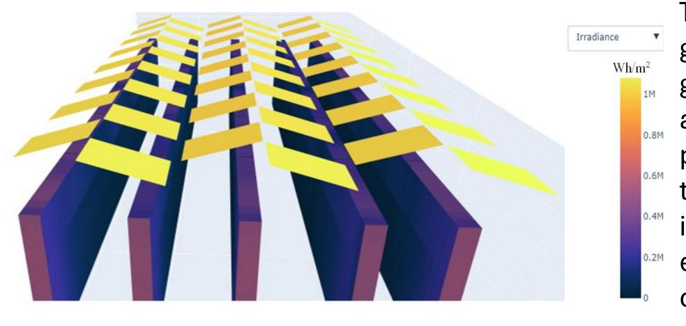
The 3D model of the east-west greenhouse includes detailed geometry of the tomato plants and PV modules, with glass properties set to 85% transmittance and a refractive index of 1.5. Irradiance was evaluated on seven key zones of the plants and modules.
